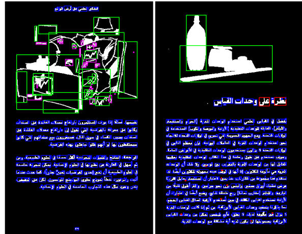
Figure 2. Examples of RFAAD performance on two images in the validation dataset. The green bounding boxes represent the non-text CC correctly classified as non-text. The blue bounding boxes represent the text CC correctly classified as text. The red bounding boxes represent the text CC mistaken for non-text. The magenta bounding boxes represent the non-text CC misclassified as text.
