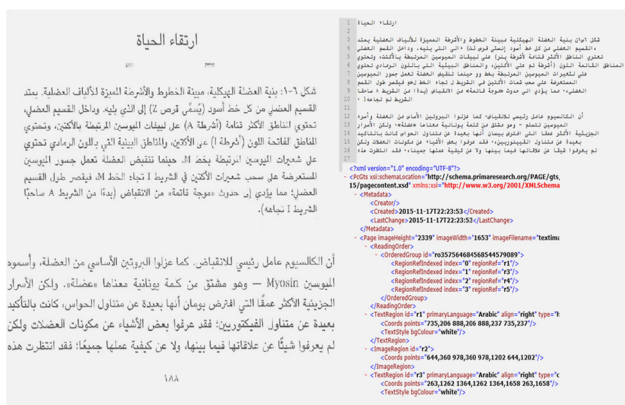
Fig. 5 Sample output of our ECDP system: extracted text zones (left), Tesseract OCR output (upper right), and XML file (lower right)
