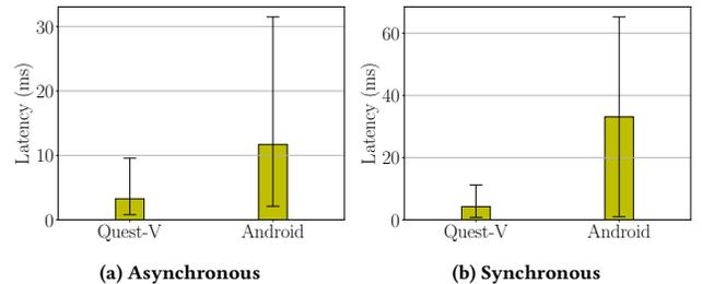
Figure 4: Average I/O Latency (min-max as error bars)
