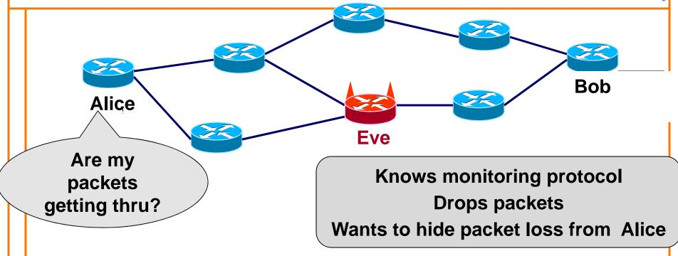
Today's approaches cannot withstand active attack (ping, traceroute, active probing, marked diagnostic packets)
