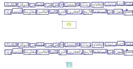
Fig. 3. Dependence of the classification of the neural network on the precision of human annotation of the training data. If the human annotator draws the border of the page number with additional white space (top) versus snug around the characters (bottom), the network confuses the page number (cyan) for a caption (yellow).
